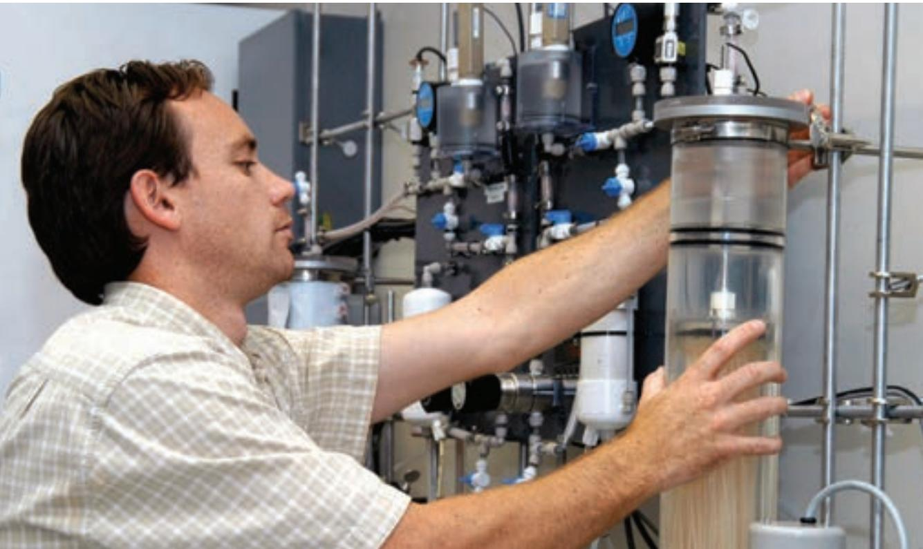
Bioprocess Engineer Tony Rector prepares one of the reactor vessels on the Aerobic Rotational Membrane System (ARMS) bioreactor for initial testing in the Space Life Sciences Lab. ARMS was designed to help treat wastewater onboard the ISS by using beneficial bacteria, which rely on a stable supply of gaseous oxygen to thrive.
